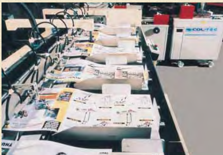
Refurbished 6 station SRA3 collator and stitch/fold/trim line installed at customers premises, overall dimensions 390 x 110 cms
